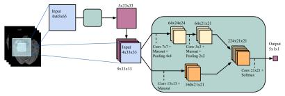
(a) Cascaded architecture, using input concatenation (INPUTCASCADECNN).
