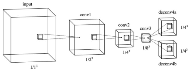
Fig. 2. A sample illustration of the 3D FCN structure used in this paper. Feature maps are first down-sampled by three convolution operation with the stride of  $1/2^3$  and then up-sampled by the deconvolution operation of the same stride. The output objectness map ( $\sigma^o$ ) and bounding box map ( $\sigma^b$ ) are collected from the deconv4a and deconv4b layers respectively.
