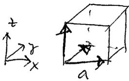
$$\begin{aligned} \vec{a}_1 &= a\hat{x} \\ \vec{a}_2 &= a\hat{y} \\ \vec{a}_3 &= a\hat{z} \end{aligned}$$
