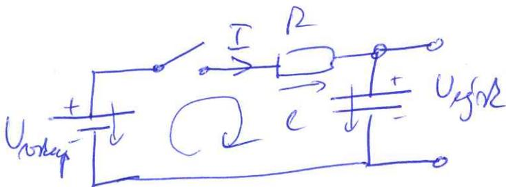
$$\oint \vec{E} d\vec{l} = 0 \quad -U_{\text{nap}} + RI + \frac{1}{C} \int_{-\infty}^t I dt = 0 \quad \left| \frac{d}{dt} \right.$$
